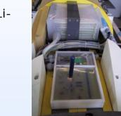
encapsulated pressure-tolerant rudder positioning sensor (magneto resistant angle sensor)
